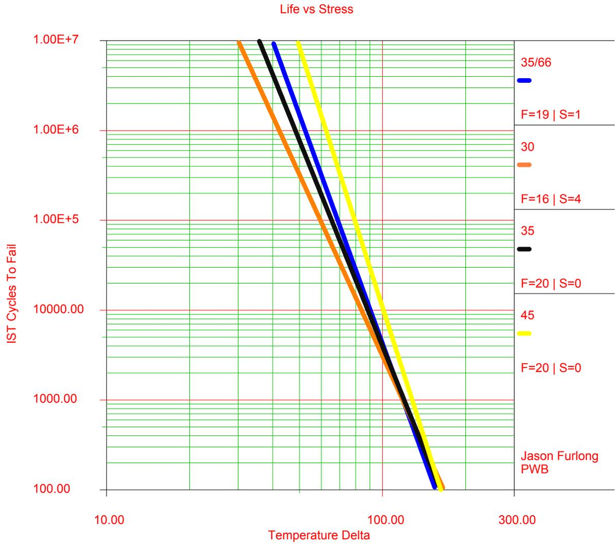
The above Life Vs Stress in graph 1, show a comparison of all four design configurations. An analysis of the graph shows that the performance order is, from best to worst, coupon 45, 35/66, 35 and 30. This result follows both aspect ratio and the pitch size, in an expected manner. However we also see that at high stress levels, about 130 (~150°C) the data starts to converge for these samples, emphasizing the need for acceleration factor analyses.
