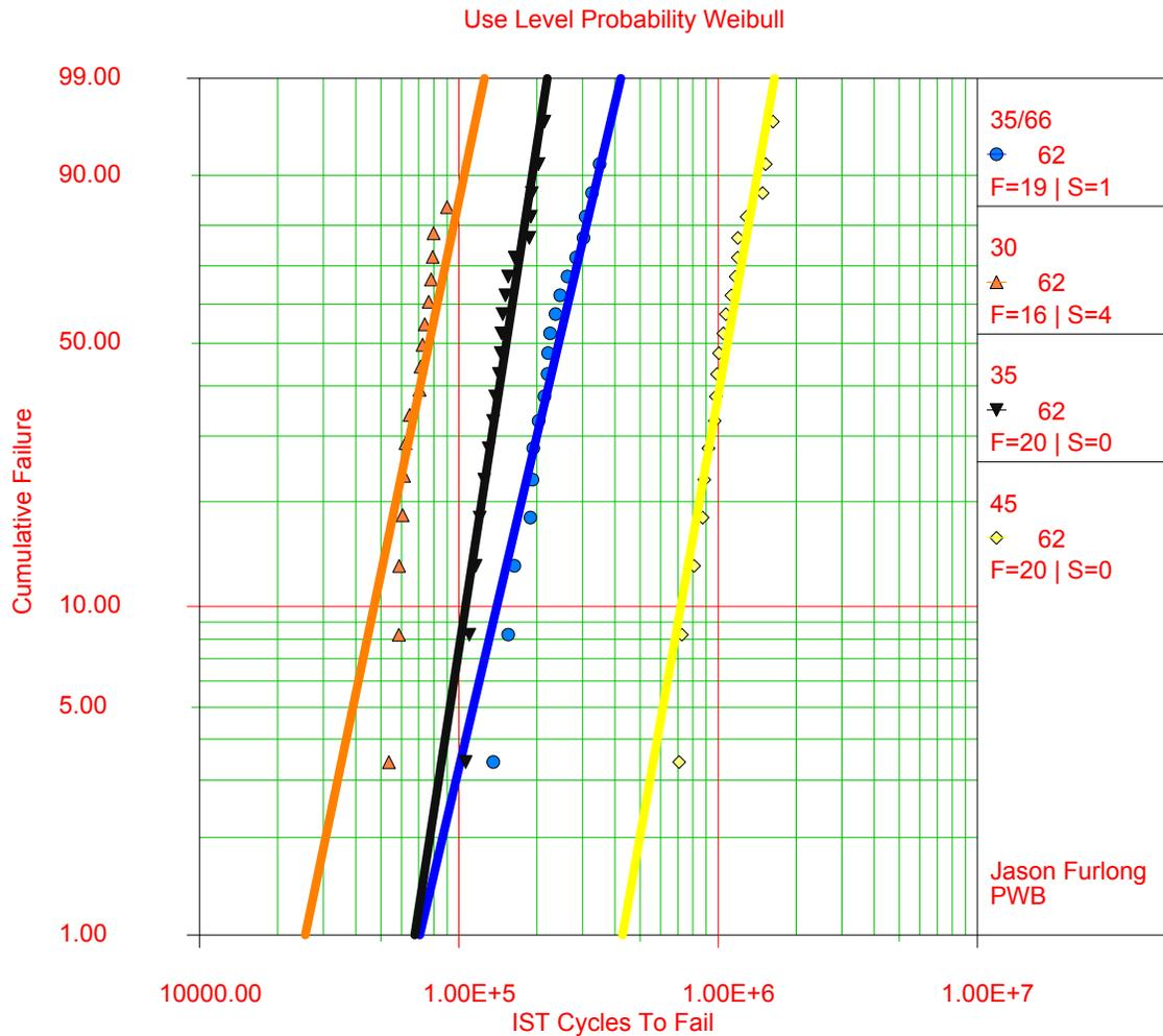
Again A visual analysis of the graph shows that the performance order is, from best to worst, coupon 45, 35/66, 35, 30. This result also follows both aspect ratio and the pitch size, in an expected manner. As can also be seen the data points are a good fit to the line of fit.
